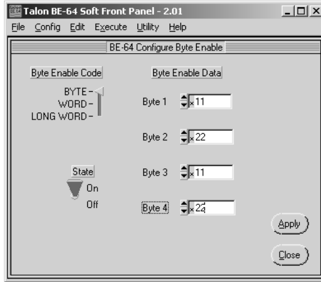
Figure 6-17 Setting Byte Enables for BYTES
